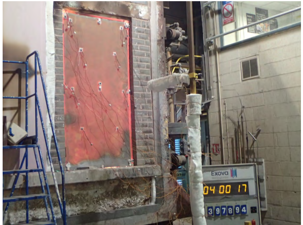
The unexposed face of Doorset B after a test duration of 240 minutes
