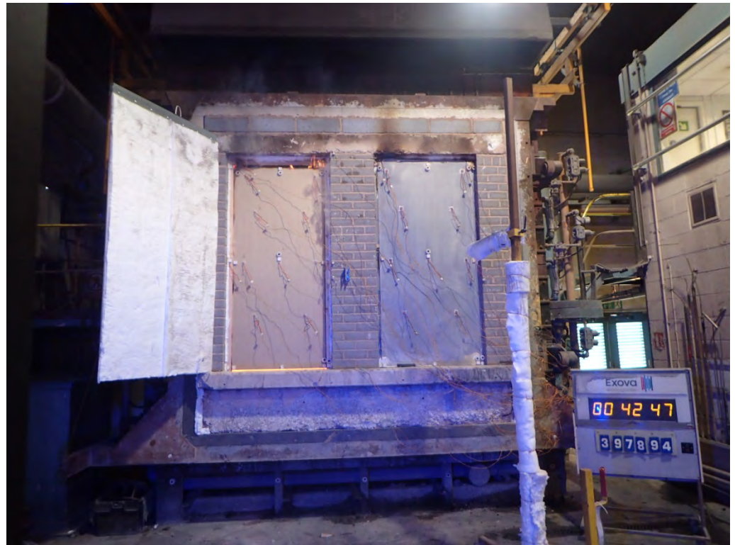
Flaming seen in the top leading edge corner of Doorset A after a test duration of 42 minutes
